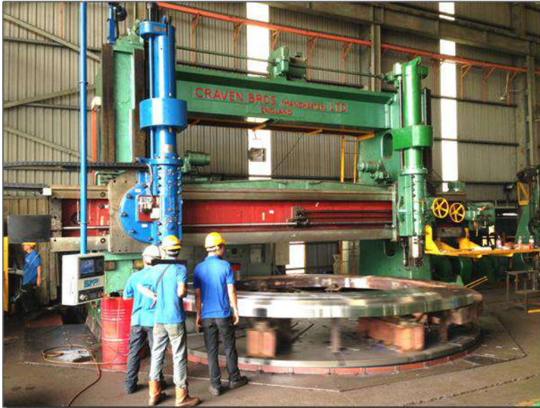
CNC- 18 FT CRAVEN VERTICAL LATHE TURNING & BORING MACHINE
