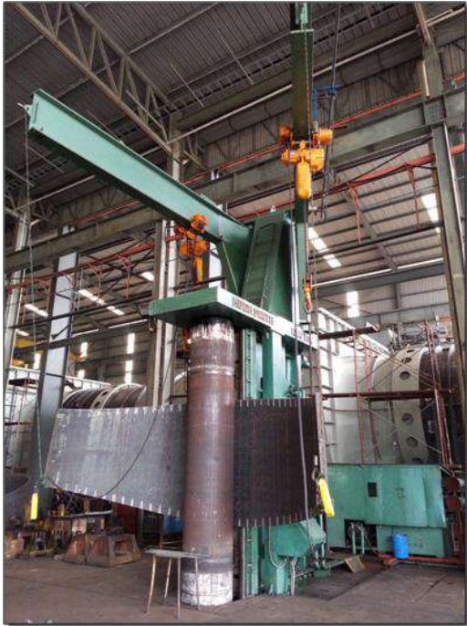
HUGH SMITH 1200 TONS VERTICAL PLATE ROLLING MACHINE
