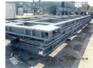
Settler Flash Furnace: Grillage Beam (26.800 kg)
