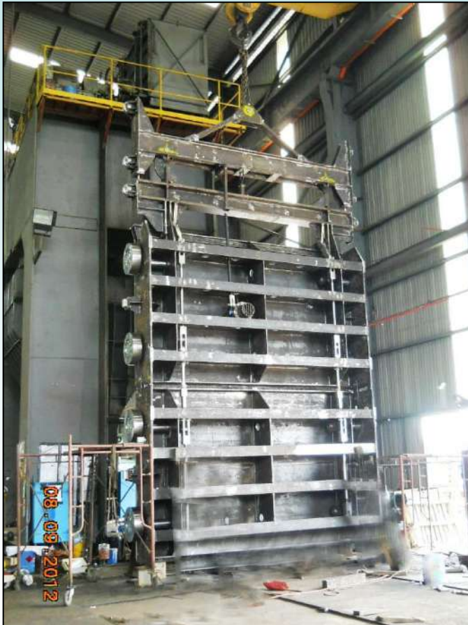
Diversion Tunnel Stoplogs -Completed Oct 2012
